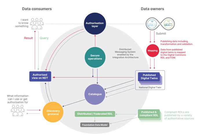
Figure 2: Conceptual View of the NDT – A National Digital Twin enabled by an Information Management Framework
