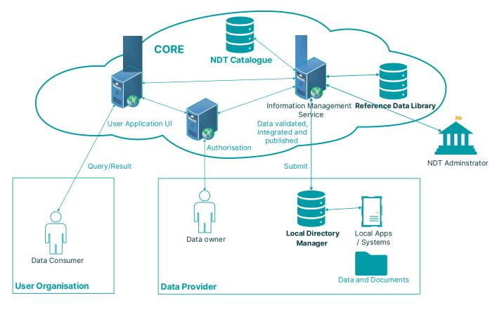
Figure 5: Centralised Architecture Pattern
