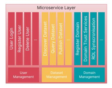
Figure 4: Microservice Layer with example services
