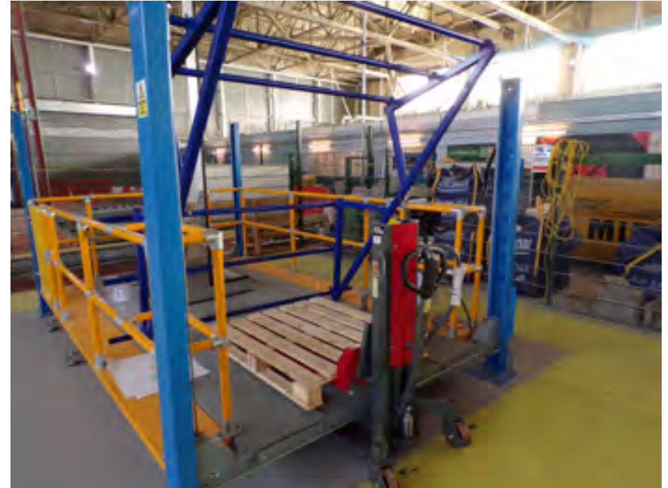
Modified car lifting jack, used to create a safe working platform for operatives stacking Superblocks - see Sub Assembly case study
