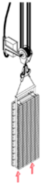
Installing facade panels (Site concrete team fill windposts)
