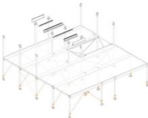
Remove props, tables + temp. bracing in remaining bays
