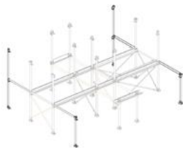
Column and edge beam installation GL 1&4/A&D
