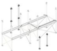
Adjacent central columns and floor opening edge beams
