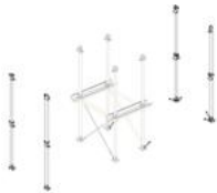
Edge columns with pre-installed brackets GL 2-3
